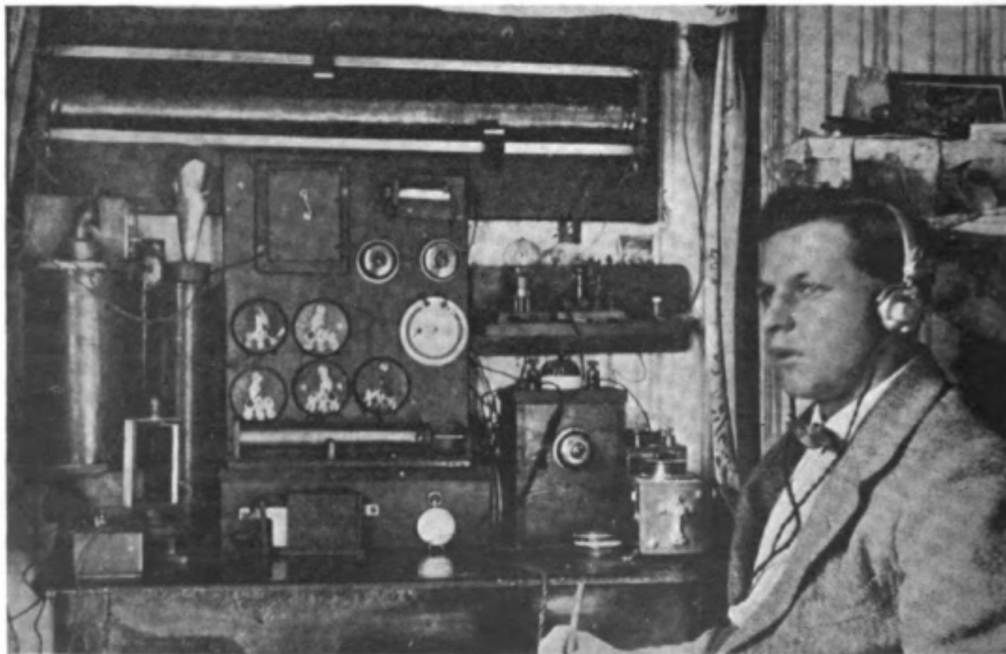
Mr. J. G. F. Harris, of Gloucester, and his wireless set, all home made except valve, telephones and power units.
